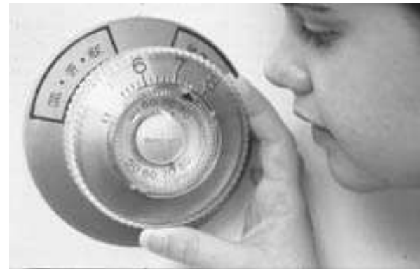
A person with low vision operates at close range a round thermostat with large numbers, tactile indicators, and audible cues.
